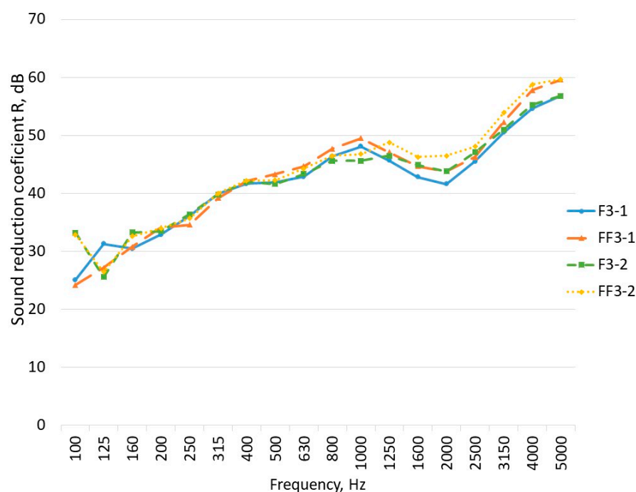
Figure 11. Comparison of dependence of sound reduction index (R) on frequency of 2nd group C type specimens (external and internal laminated glasses and inner ordinary glass). Façade element (marked with letters FF) frame cavities filled with gypsum fibreboard and empty frame (marked with letters F) (see Tables 2 and 3).
