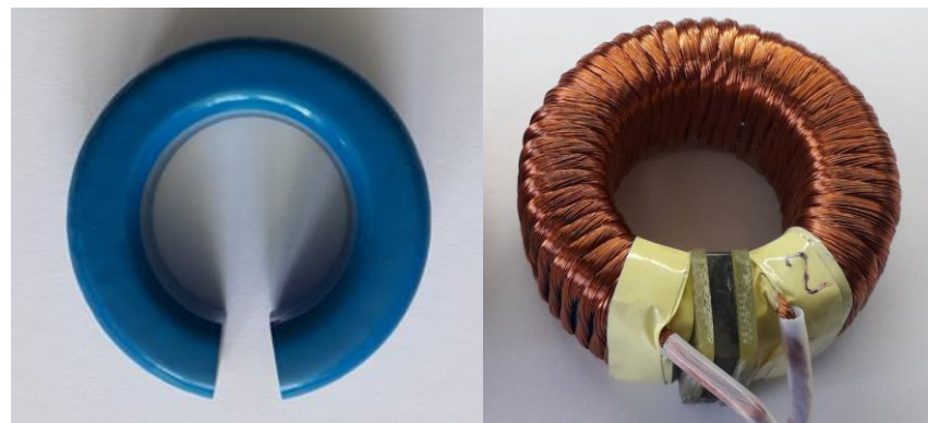
Figure 10. Alternative of the toroidal inductor with air gap given by product type (left) and modification by shortening airgap by ferrite material inserted within air gap (right).
