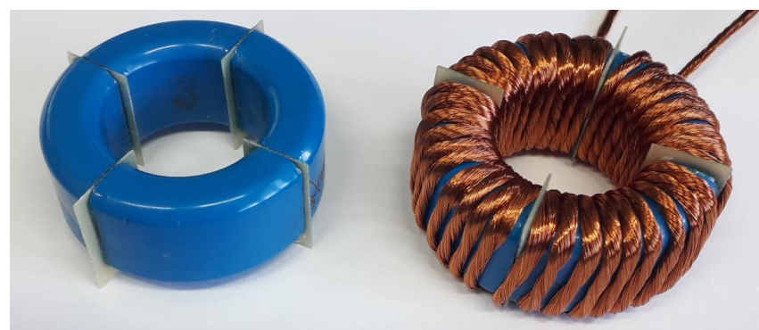
Figure 11. Alternative of the toroidal inductor with the distributed air gap without winding (left) and with winding (right).
