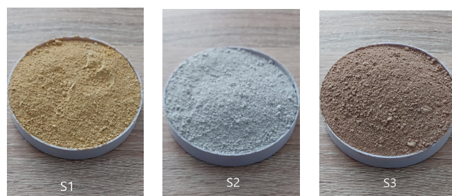
Figure 1. Clay samples in powder form: S1–clay raw material from a deposit in Germany, S2–clay raw material from a deposit in Estonia, S3–clay raw material from a deposit in Lithuania.
