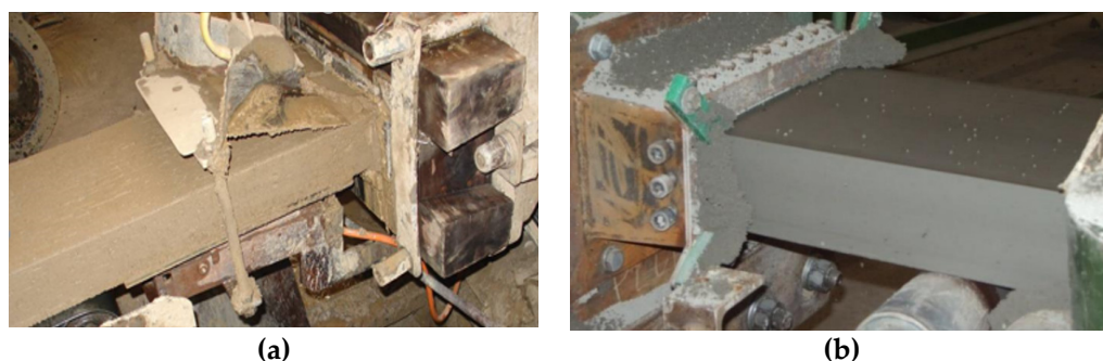
Figure 3. Clay extrusion process: (a) extruded bar of clay S2, (b) extruded bar of clay S3.
