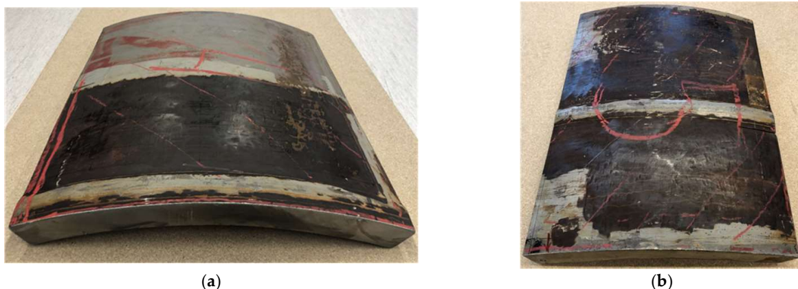
Figure 1. Segments of heat exchanger pipe used for comparison of HTHA detection algorithms: (a) sample no. 4 and (b) sample no. 5.
