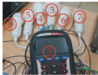
Figure A2. Photo of experimental setup for the reactive power provided by LED devices analysis.
