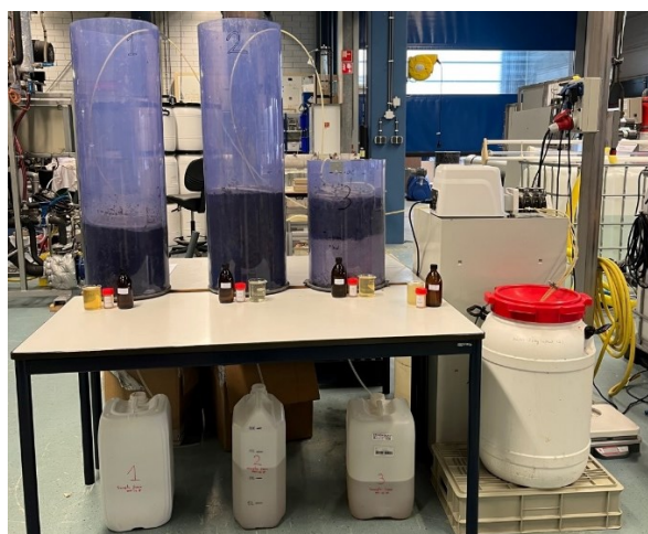
Fig. 13. Lab-scale setup for biofiltration experiment
