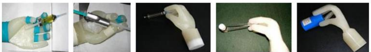
Fig. 13. Created wax phantoms in different positions for dose simulation [60]
