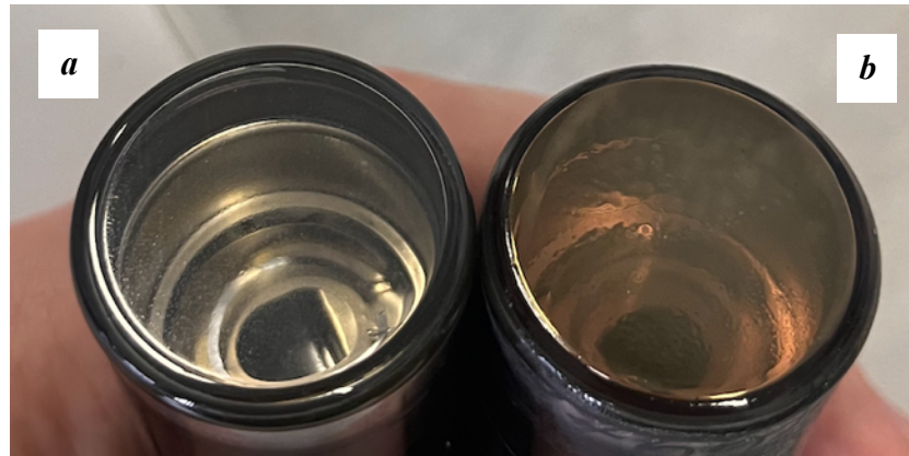
Fig. 23. Broken photocathode of the PMT (a) and unbroken (b)
