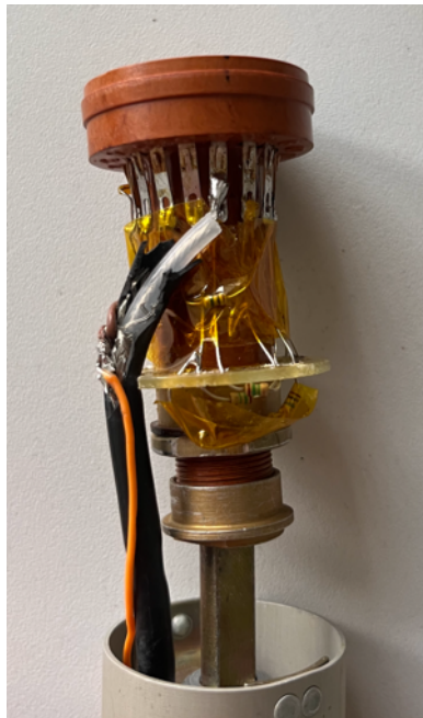
Fig. 25. New voltage divider circuitry for \phi_{3y} - 85
