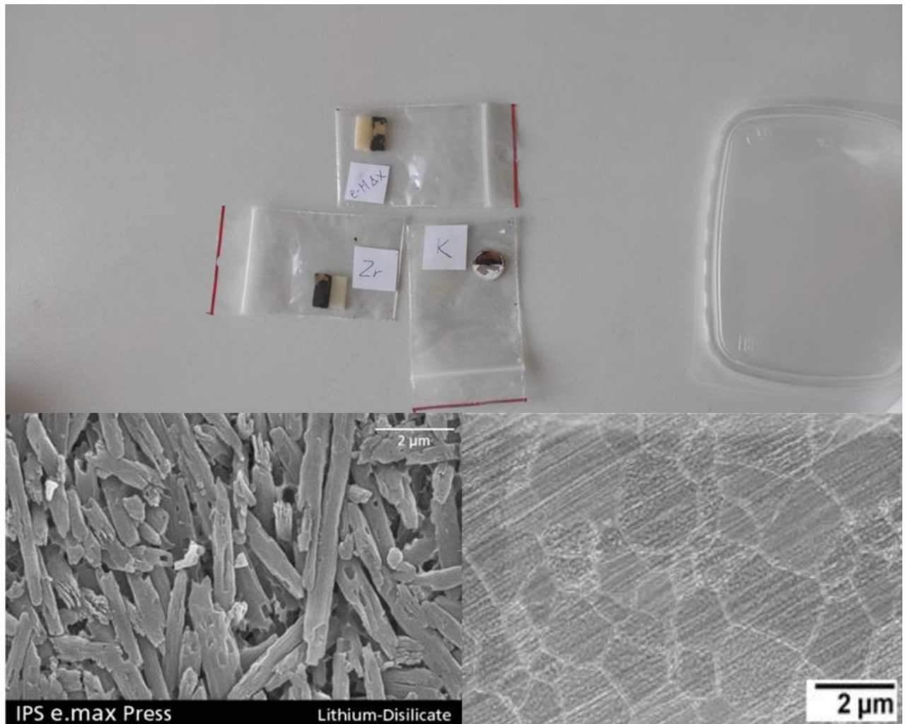
Figure 5. Upper image: Ivoclar Vivadent IPS E.max press (E-max), Katana Zirconia STML (Zr) and ENAMEL plus HRi biofunction (K) samples; Image on the left: E-max sample atomic force microscopy image [99]; Image on the right: Zr sample atomic force microscopy image [100].
