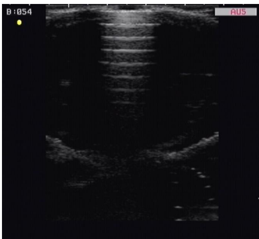
Figure 9. US imaging of Zr sample in water with 7.5 MHz probe
