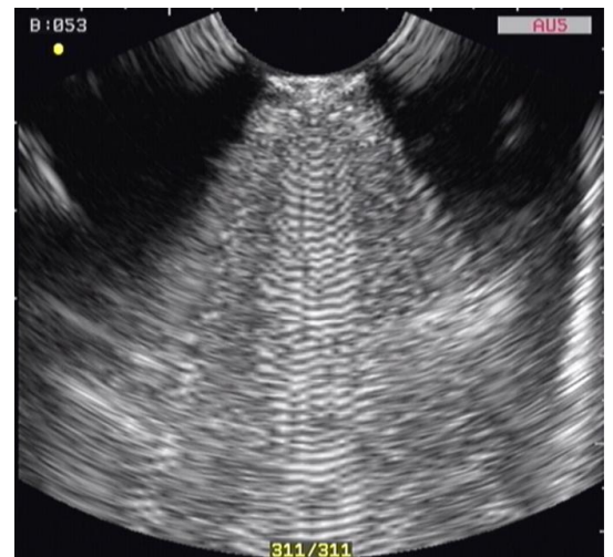
Figure 18. US imaging of Aluminium ( Al ) sample in water with 6.5 MHz probe
