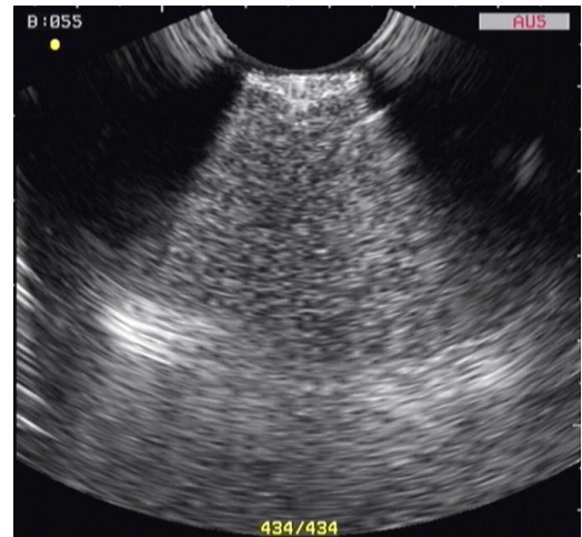
Figure 10. US imaging of Zr sample in water with 6.5 MHz probe
