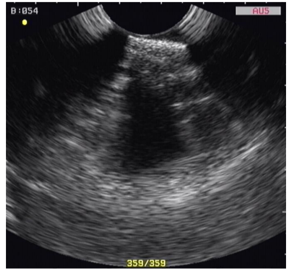
Figure 14. US imaging of K sample in water with 6.5 MHz probe
