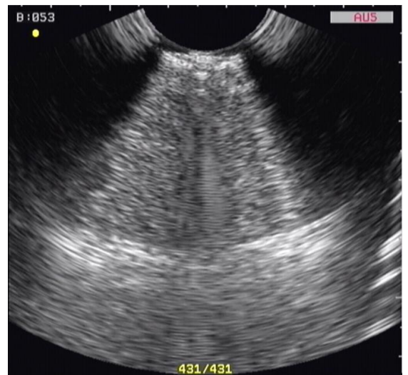
Figure 16. US imaging of E-max sample in water with 6.5 MHz probe
