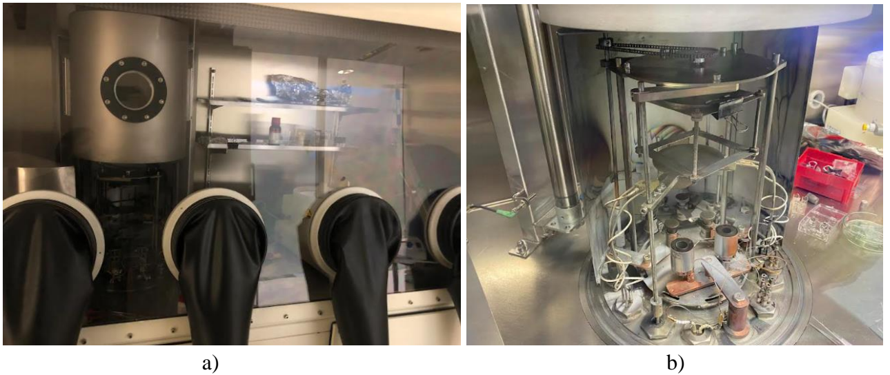
Fig. 24. MB EcoVap4G glove box containing (a) Kurt J. Lesker vacuum deposition chamber (b)
