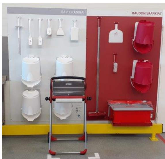
Fig. 20. 5S shadow board for contacting (white) and not contacting tools
