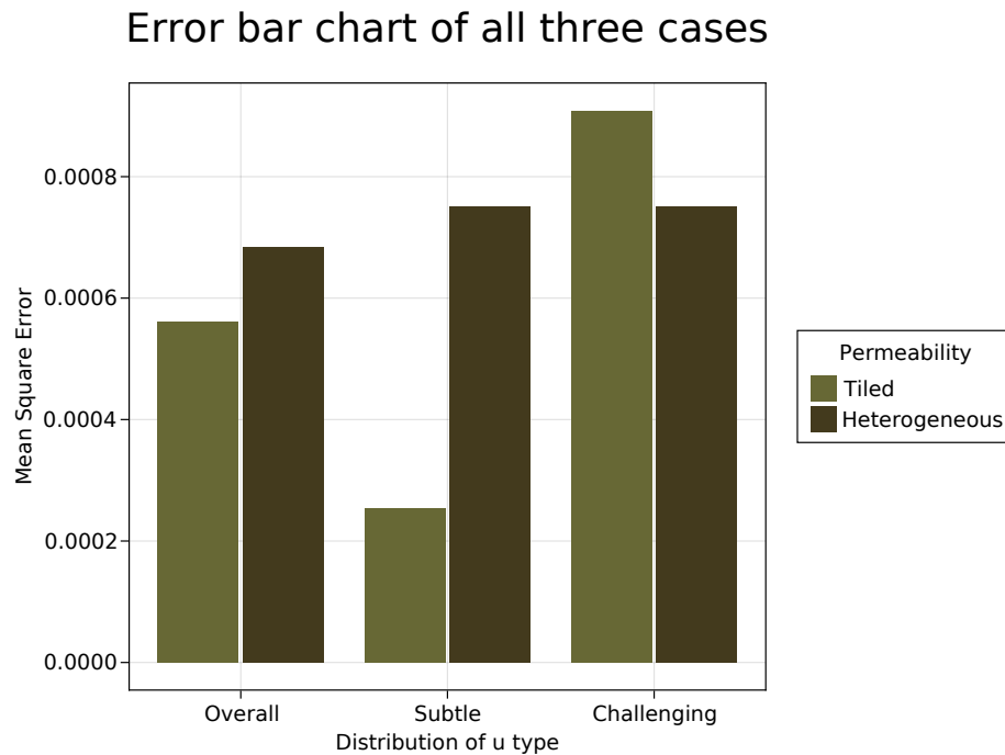
Figure 3.10: Bar chart depicting an average of each u distribution case MSE between FVM and CDNN. For each permeability (tiled/heterogeneous) there were three distinct u distribution types - a type for somewhat uniform u distribution over the domain where one colour dominates over all, a type for more subtle shapes in the solution and a type for challenging cases.
