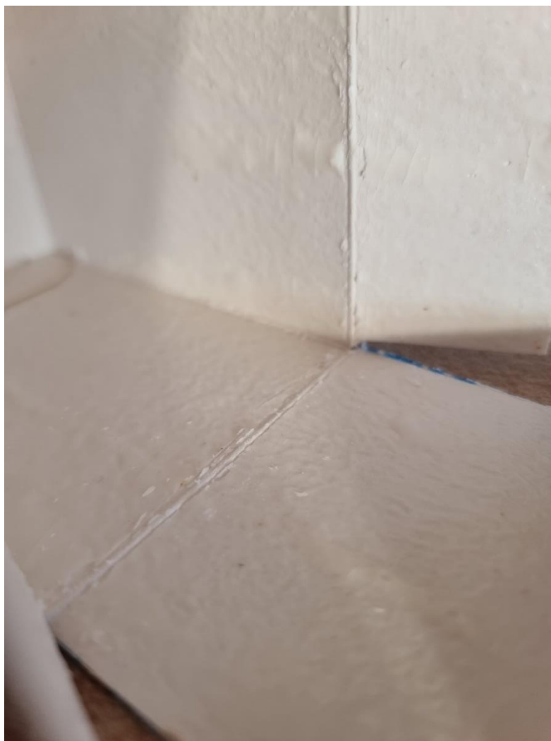
Fig. 21. Wax coating after folding on the paper box surface
