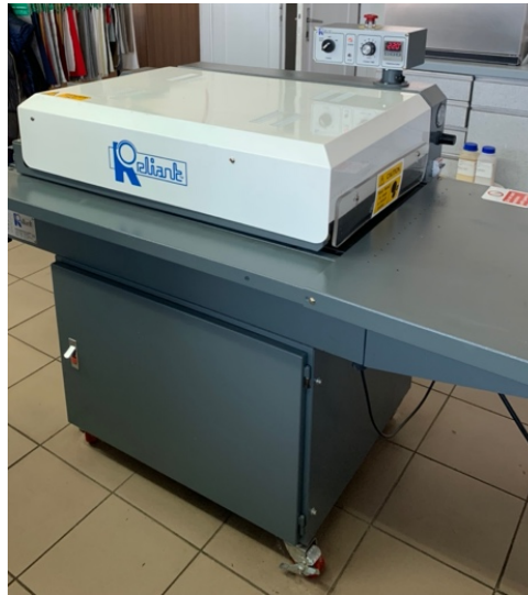
Fig. 13. Nova-45 (Reliant Machinery, Ltd., United Kingdom) fusing machine
