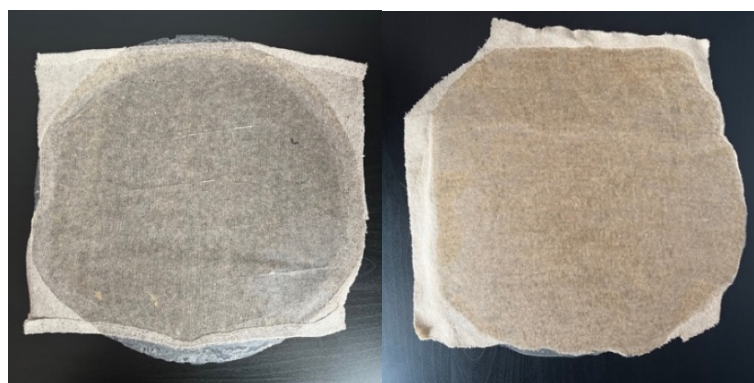
Fig. 12. Produced knitted hemp fabric/PLA composites, Felina 32 fabric/PLA – left, USO 31 fabric/PLA – right
