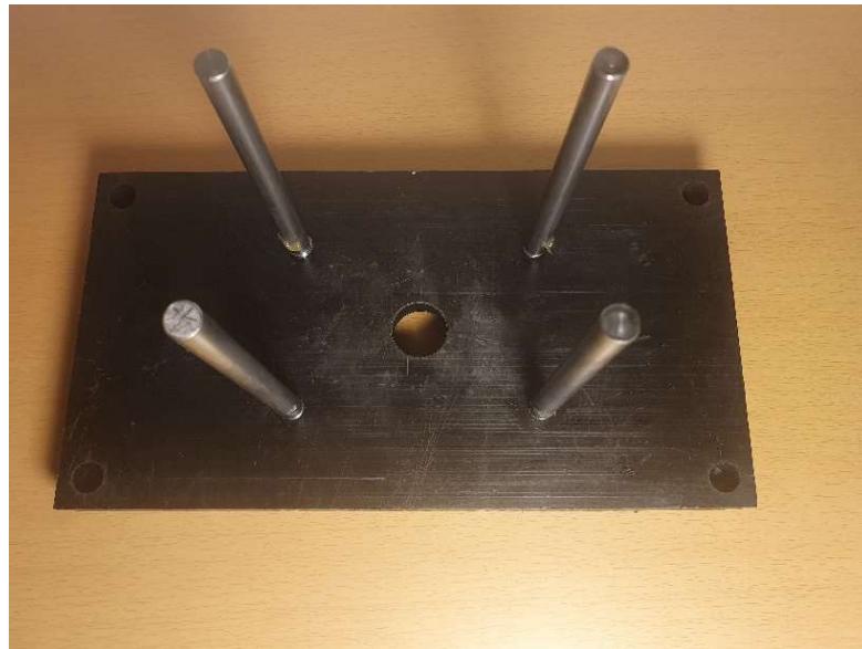
Fig. 23. Top housing with linear guides
