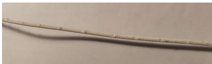
Fig. 32. 9wt% PVDF/BaTiO 3 filament after feeding to 3D printer extruder
