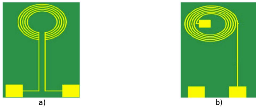
Fig. 11. Micro electromagnetic coils analyzed by Majlis et al. [29]: a) parallel planar circular coil; b) spiral planar circular coil
