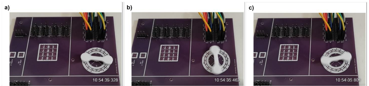
Fig. 33. Screen captures of a video demonstrating 120rpm rotary motion, starting at image a)
