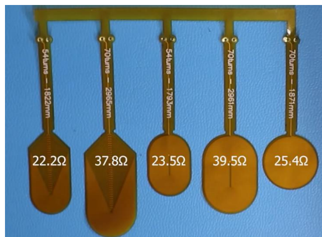
Fig. 14. Coil topologies of new PCB coil actuators by Carl Bugeja [31]
