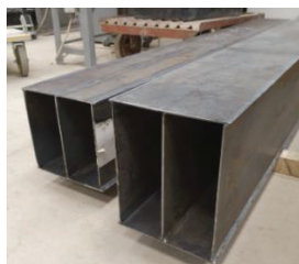
Fig. 2.9. View of experimental beams prior to concrete casting
