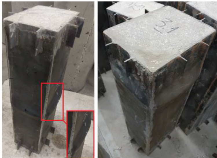
Fig. 2.3. Experimental column post-buckling shapes
