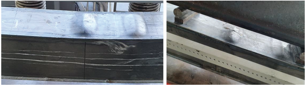
Fig. 2.12. Experimental post-buckling shapes of beams
