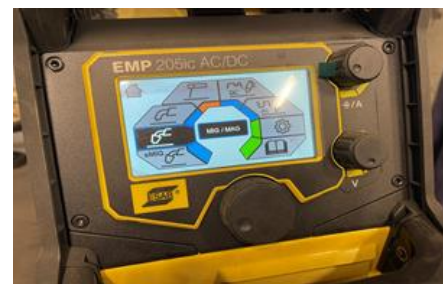
Fig. 3 Interface of ESAB REBEL EMP 205ic with selection of welding processes
