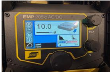
Fig. 4 Automatic selection of welding parameters
