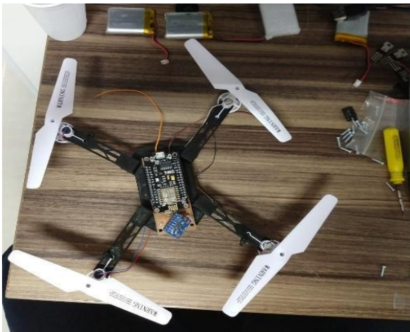
Fig. 3: Drone's parts printed in 3D
