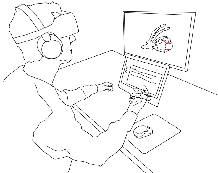
Figure 6. Setup for multi-sensory learning. The user wears a head-mounted display to get access to the visual contents. He also wears wearable haptic interfaces in their right hand reproducing tactile cues.
