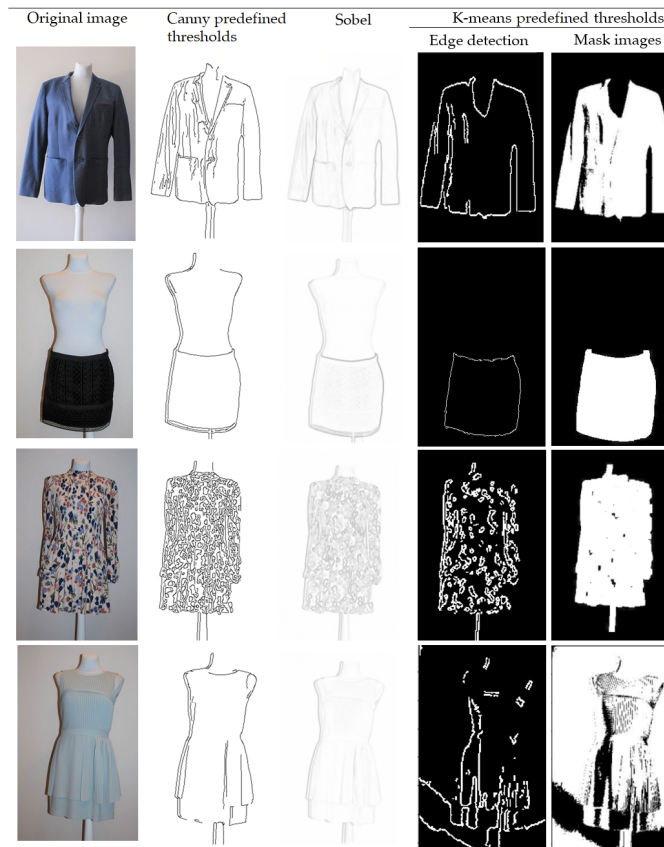
Figure 3. Results of different contour detection techniques: Canny algorithm with predefined threshold values, Sobel algorithm and K-means based thresholding algorithm providing edge and mask images.
