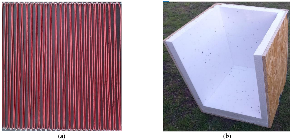
Figure 1. Preparation of laboratory setup: (a) arrangement of the heating cable; (b) thermal insulation of the setup.
