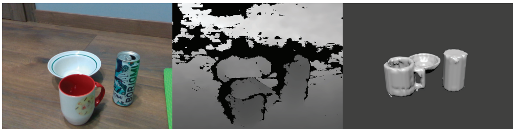
Figure 15. An example of reconstruction of multiple objects in the scene: segmented and classified RGB frame ( left ), depth frame ( middle ), and predicted depth mask ( right ).
