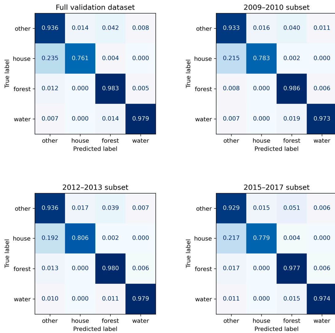
Figure 9. Normalized confusion matrix of M123 segmentation results for full fine-tuning validation set and its subsets of different periods.
