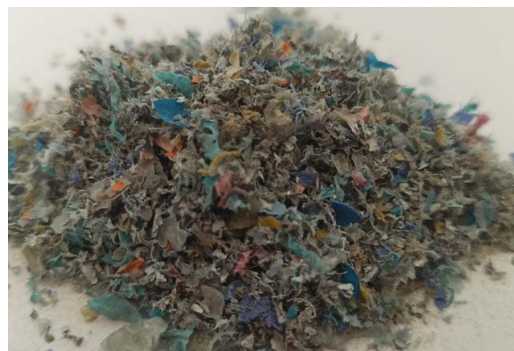
Fig. 2. SRF produced from RDF
