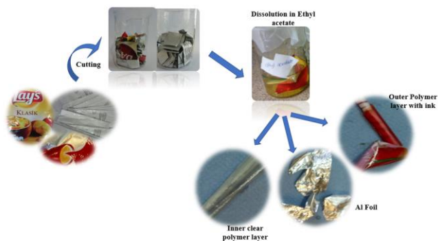
Fig. 16. MFPW Separation stages and separated (aluminum, transparent thin polymer layer, and polymer layer with unrecovered paint) by ethyl acetate [3]
