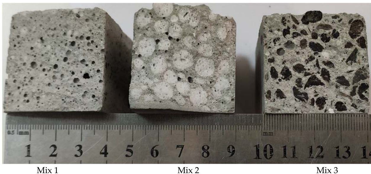
Figure 6. The macrostructure of the lightweight aggregate shotcrete samples.
