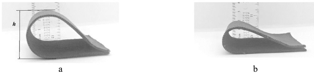
Figure 1 – Height measurement of free fold loop-shaped specimens: (a) – wale direction; (b) – course direction.
