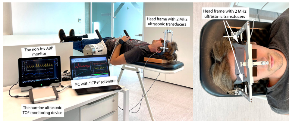
Figure A1. The CA monitoring setup includes the noninvasive ultrasonic TOF monitoring device with the head frame, noninvasive blood pressure monitoring device, and a personal computer with “ICP+” software for real-time calculation of CA index (VRx). A head frame bearing a pair of ultrasonic transducers (2 MHz) on either side of the patient’s head was positioned to transmit and receive the ultrasound wave.
