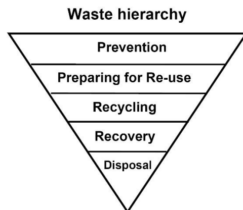
Figure 1. The waste hierarchy according to ‘the Waste Framework Directive’ of the European Union [7].
