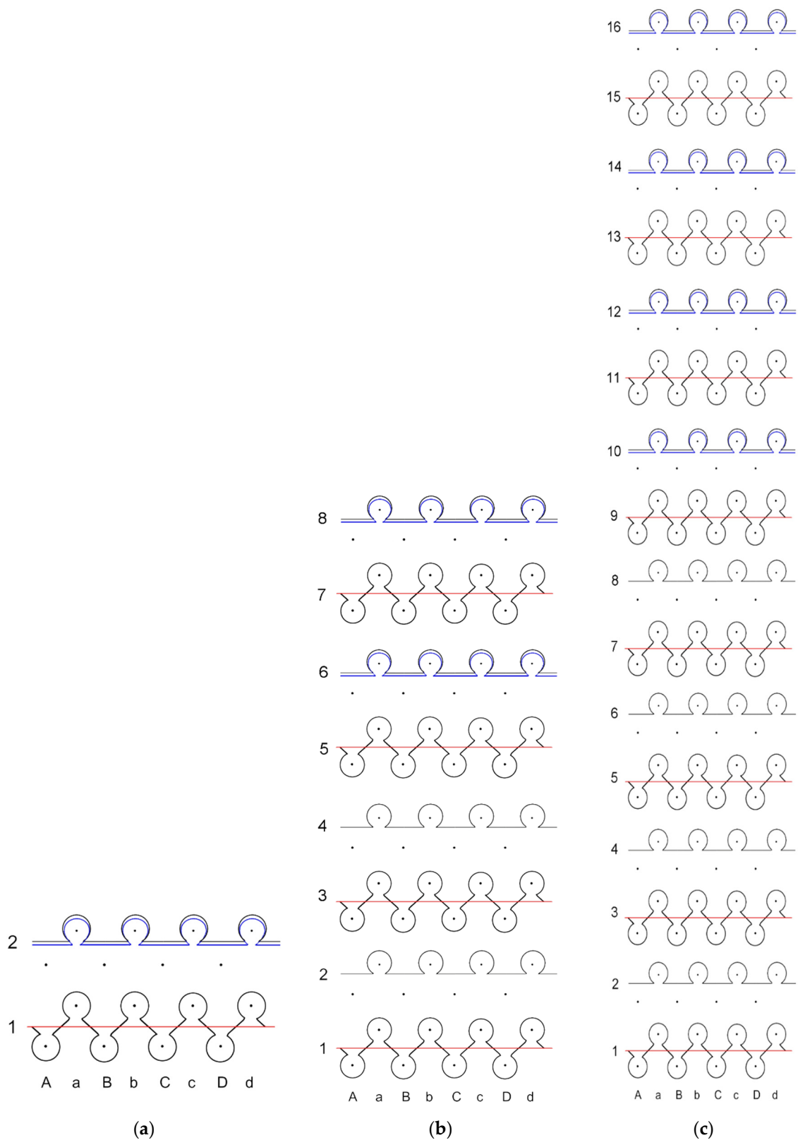
Figure 1. Principle scheme of conductive yarn layout and sample identification: (a) CF_LY1 and CF_HY1; (b) CF_LY2 and CF_HY2; and (c) CF_LY3 and CF_HY3. (○) PA6.6 ground yarn, (○) PA + Ag conductive yarn (66 tex for CF_LY and 235 tex for CF_HY), — Elastomeric inlay yarn).
