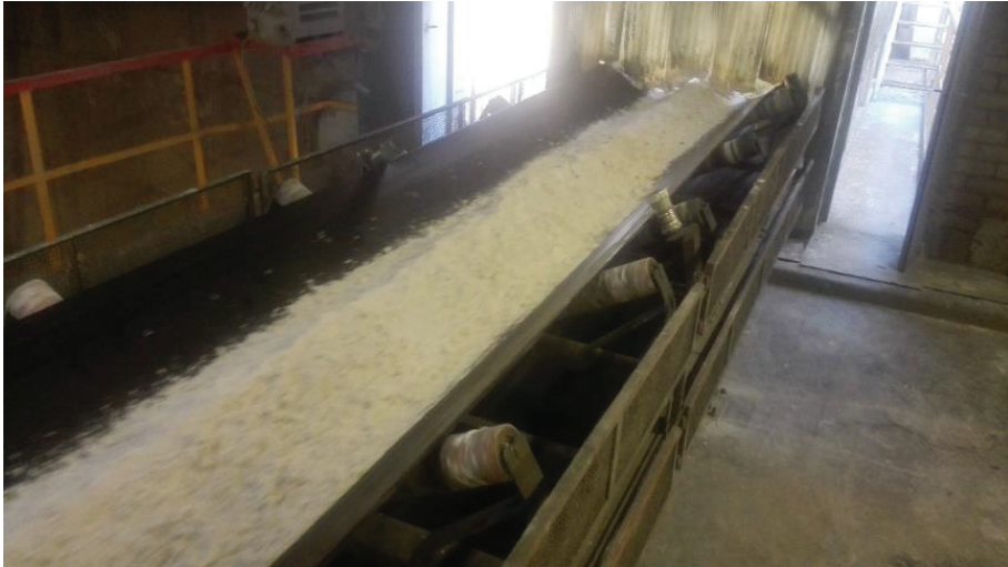
Fig. 1. View of the manufactured humid PG powder in a chemical plant of phosphate fertilisers, straight after the wet process
