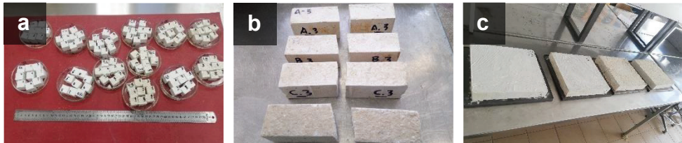
Fig. 56. Images of the manufactured specimens for different tests: 2 cm-sided cubes for CS test (a), the 4x4x16 cm prisms for FS test (already tested) (b) and 30x30x5 cm panels for measurements of \lambda (c)
