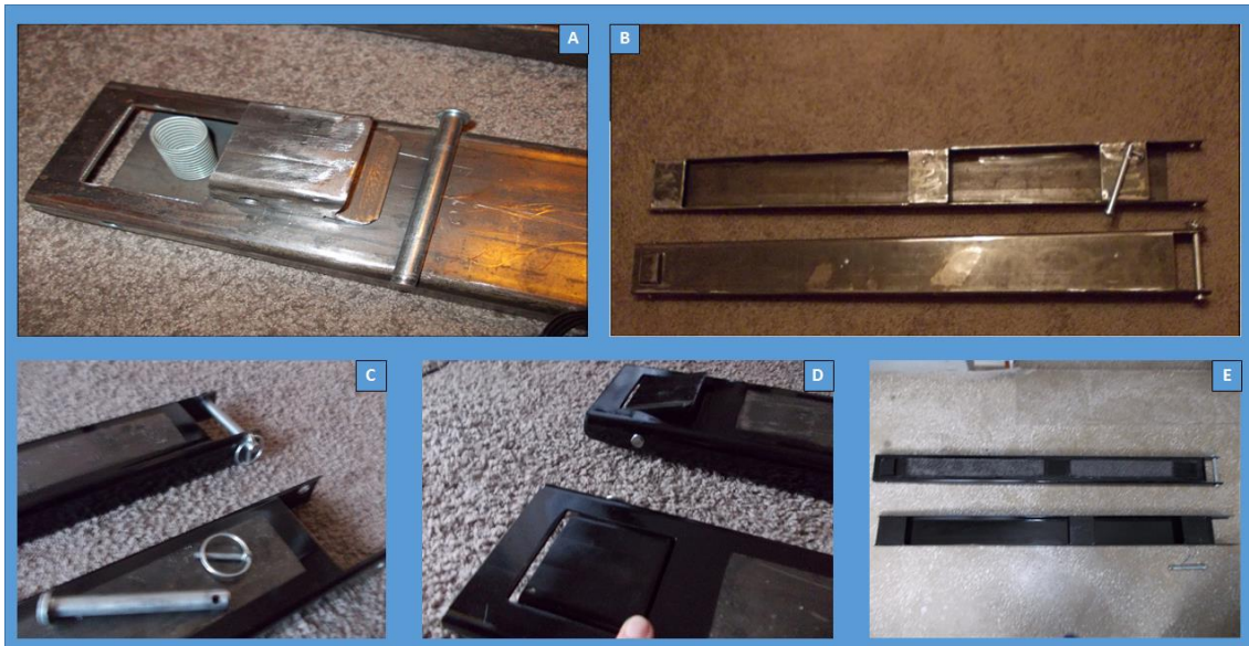
Figure 11. (A)—Locking mechanism; (B)—Fork pads in their raw state; (C)—Fork pads—fastening mechanism; (D)—Painted fork pads—locking mechanism; (E)—Ready fork pads.
