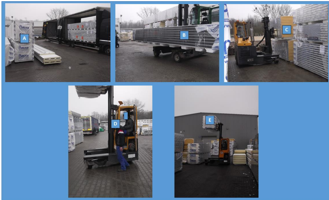
Figure 17. Transporting the load with a forklift. (A)—Pallets in the square; (B)—The pallet is transported with a forklift; (C)—The pallet is picked up by a forklift; (D)—View: forklift forks under the pallet; (E)—The forklift puts down the pallet.
