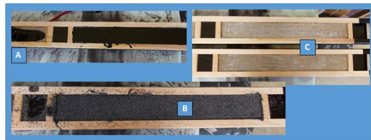
Figure 12. Technology of the anti-slip layer: (A)—Mould for casting the elastomer; (B)—Covering the elastomer with corundum; (C)—Mould for casting the elastomer.
