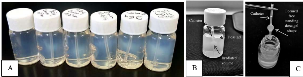
Fig. 64. A – nPAG F dose gel samples irradiated in Elekta Flexitron Icon TM in brachytherapy unit with 192 Ir source with different doses, B – example with free standing dose gel shape inside the bottle, C – free standing polymerized gel removed from the whole gel volume
