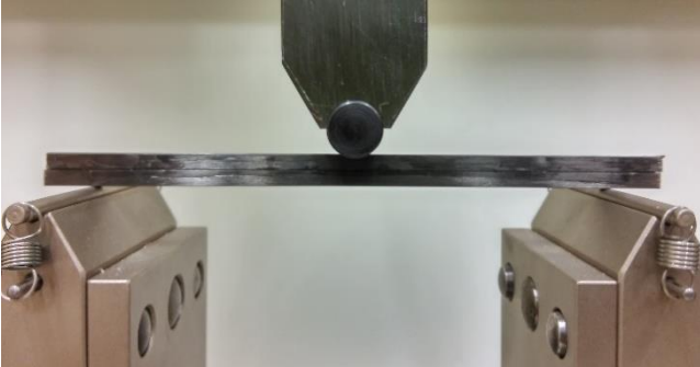
Fig. 7 Three-point bending test (Mode II)
