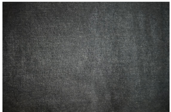
Figure 4. Photograph of developed 3/1 right-handed Z-twill denim.
