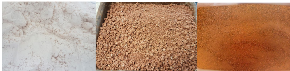
Fig. 1. Raw materials. Silica gel, unburned red clay before milling and red brick sand.
