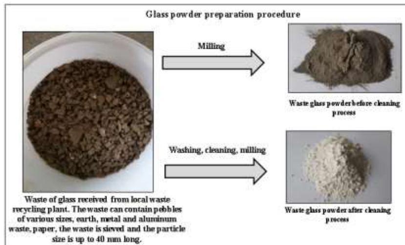
Fig. 4. Waste glass powder preparation procedure
