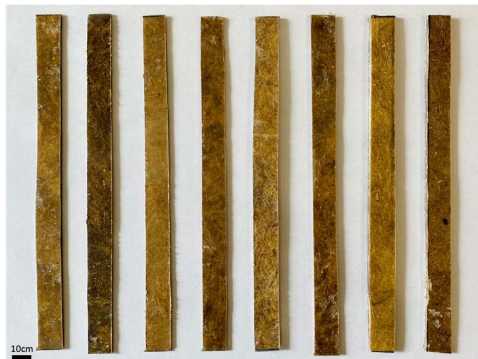
Figure 2. Prepared composite samples for the tensile test (from left: OB/P, OB/E, MB/P, MB/E, IB/P, IB/E, MR/P, MR/E).
