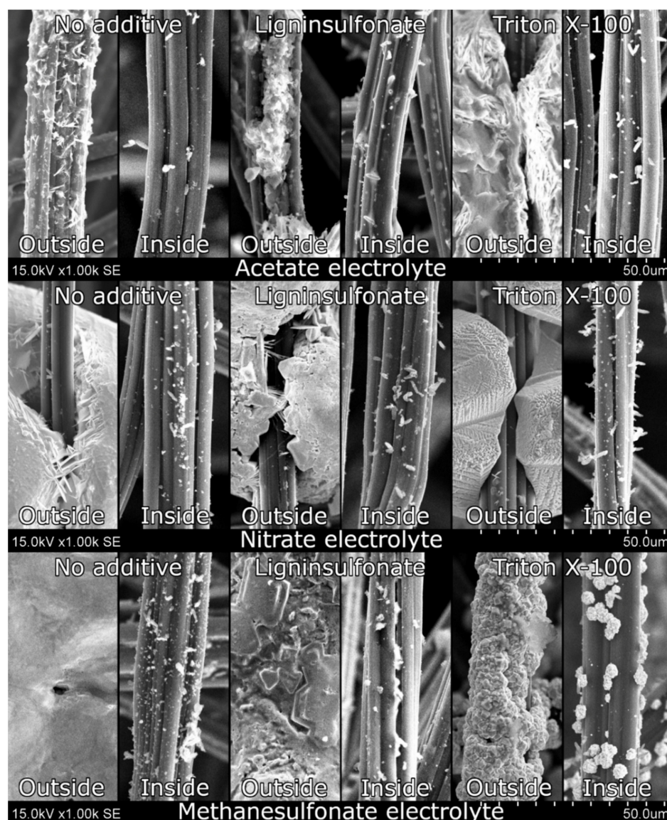
Figure 5. SEM images of samples polarized negatively during electrodeposition at 1000 \times magnification. The top, the middle, and the bottom rows show samples modified in acetate, nitrate, and methanesulfonate electrolytes, respectively. The left, the middle, and the right columns show samples modified without additives, with sodium ligninsulfonate, and with Triton X-100, respectively.
