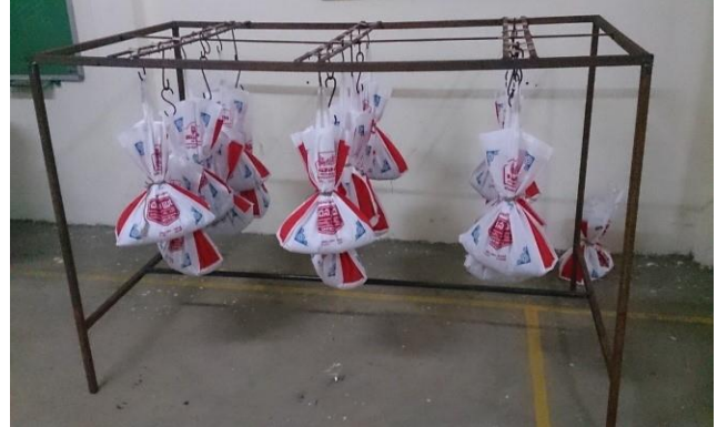
Fig. 3 Flexural creep test arrangement
