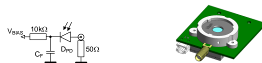
Fig. 20. Photodetector schematic diagram (left) and 3D drawing of the assembled sensor (right).
