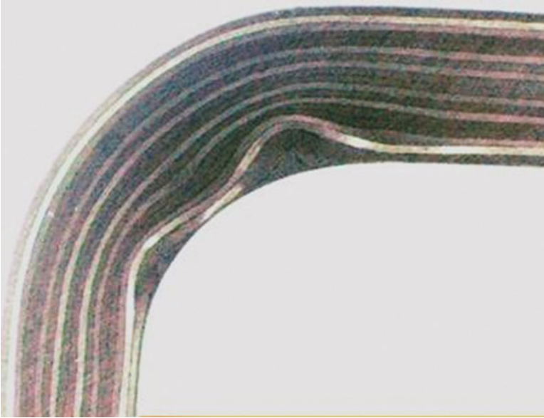
Fig. 3.38 Laminate wrinkles in composite radius
