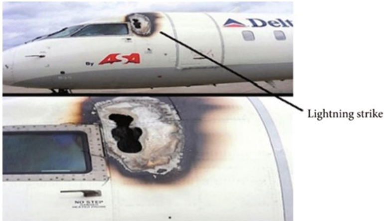
Fig. 3.21 Lightning strikes damage to a regional jet (Alemour et al. 2019)
