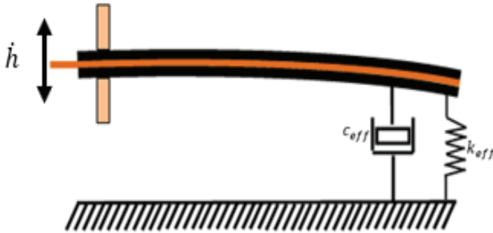
Figure 2.3. Schematic drawing of CB structure with ERF damping medium and its vibration behaviour, CB compressed
