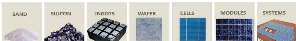
Figure 5. Production chain of silicon based photovoltaic devices (Image adapted by using information received from Soli Tek R&D)
