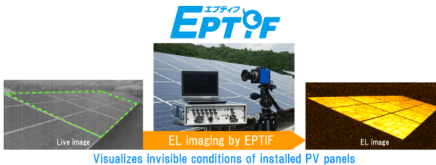
Figure 32. On-site EL/PL Inspection Machine EPTiF [40]
