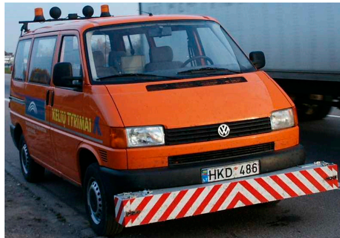
Figure 23. Laser profilograph DYNATEST 5051 RSP mounted on the VW Transporter. Reprinted from ref. [58].
