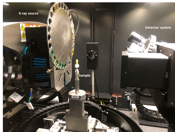
Figure 3. The general layout of the experiment including the X-ray source, the specimen, and the detector.
